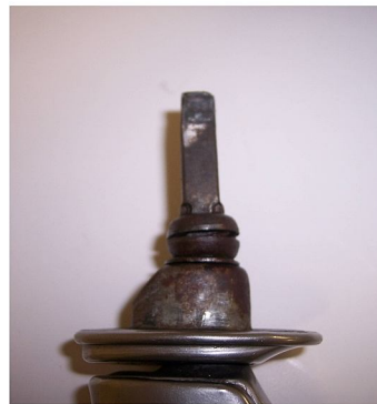
Fig. 2 File or sand shaft to size
