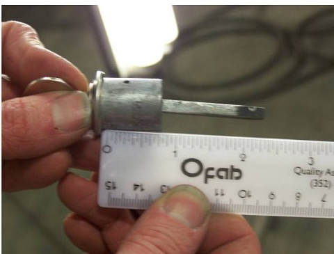
Fig. 7 Measure (Coupe) 2 1/2" or (Tudor) 2 1/16" from base with no gasket. Mark and cut shaft. If you are using a gasket you will need to add the gasket thickness to the length of the shaft.
