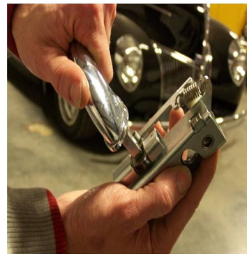
Fig. 2a Test fit shaft to latch
